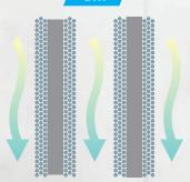
The fan operation after shut down helps dry water droplets to keep the coils dry and clean
